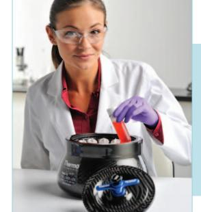
Rotor selection is critical when it comes to sample safety and centrifuge performance. Thermo Scientific™ Fiberlite™ carbon fiber rotors are designed to deliver exceptional performance without fatigue or corrosion for worry-free operation spin after spin.
