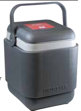
• 27211 PROFESSIONAL VACCINE CARRIER Compact, extra strong with special insulation by high density PU foam suitable for transportation of vaccine. Comes complete with 8 empty ice-packs 400 ml suitable for a cold life of 40 hours at 8°C with external temperature of 43°C without opening. Vaccine storage capacity: 2.6 l. Body and lid with gaskets for better insulation. External size: 28.5x25.5xh 32 cm. Internal size: 22x18xh 24 cm. Made in Italy.
